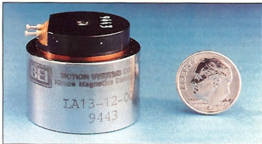
Figure 1 — Linear voice coil actuator with the copper coil wound around a ferromagnetic cylinder. Two wires connect to the coil leads, shown above the coil winding.
