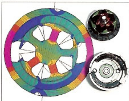
Fig. 2. Disassembled 24V cordless power tool motor and a magnetic flux contour plot of the motor cross-section.
