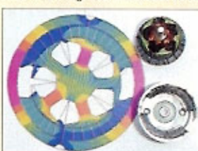
Figure 1. Rotor and stator of a d.c. appliance motor, with FEA flux distribution at rated output.
